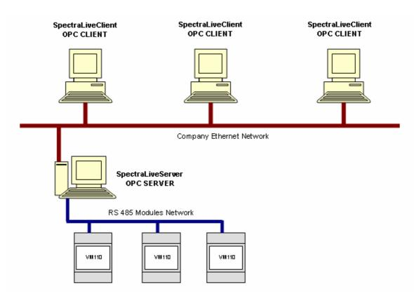
All the VM110 Modules are connected to a single computer (named here Server).
